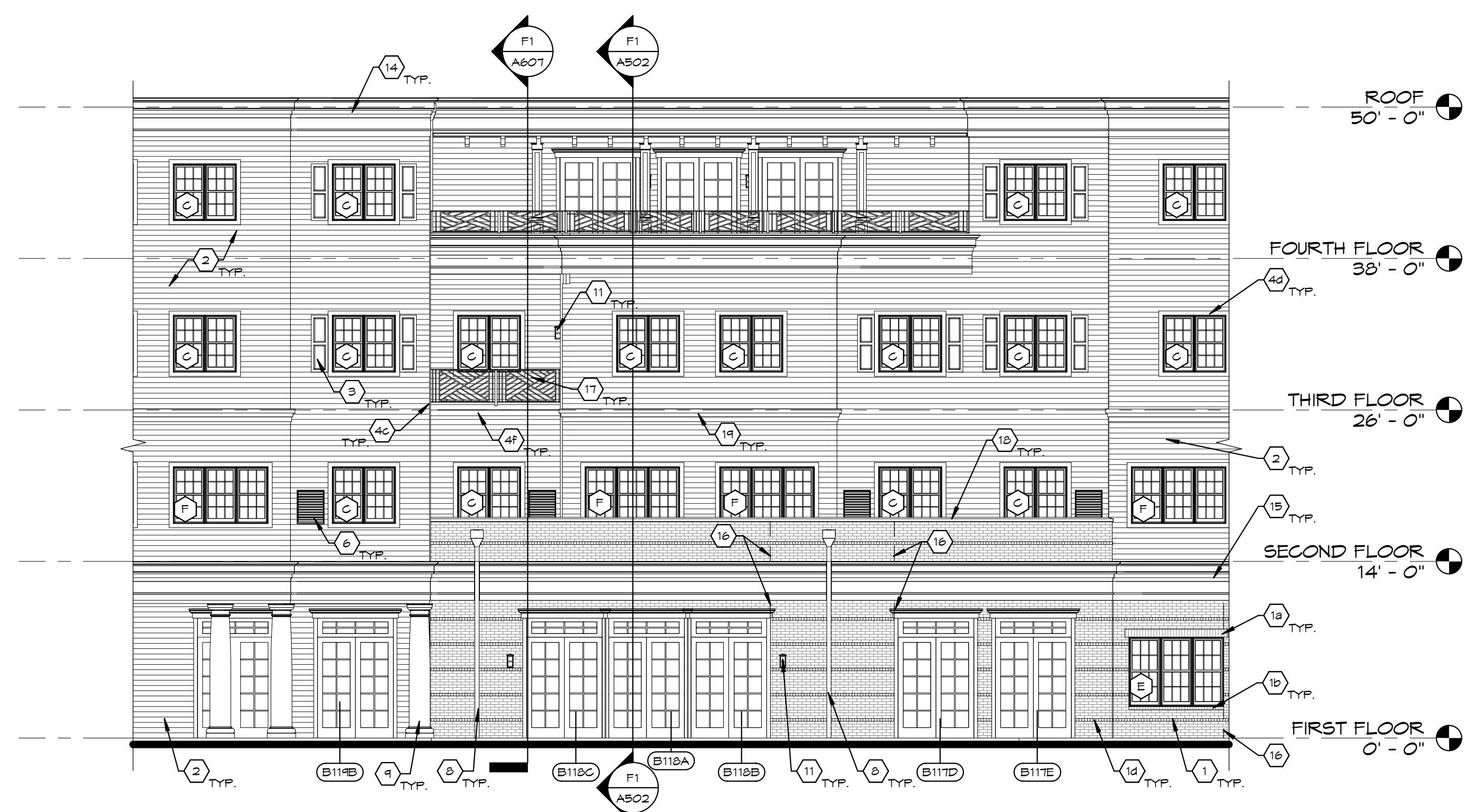
F2 PARTIAL REAR ELEVATION (EAST) 1/8" = 1'-0"
